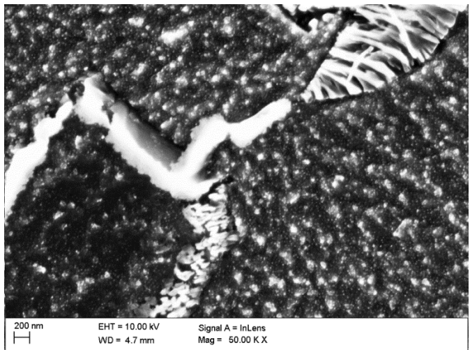
Figure 15: SEM images (InLens mode) using Hydrochloric-Nitric-Acid (6:1) etching after an aging of 5000 h at 600°C.
